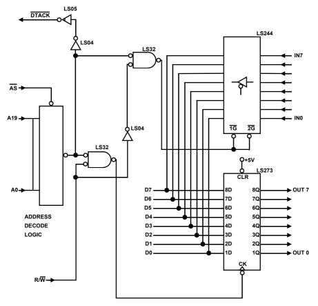
This circuit works satisfactorily on my 68008 system, so I would expect it to work on the QL, with appropriate logic for the address decoding. I seem to remember that the QL should have all the I/O devices in the top 64K of the memory map.
